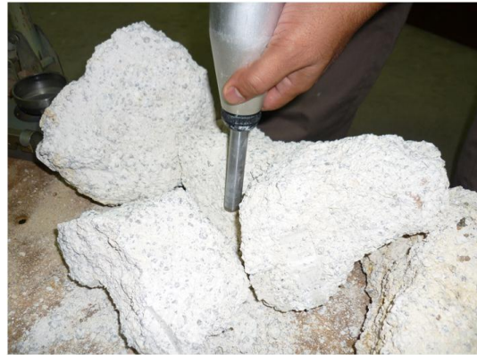
Fig. 7 The sample was destroyed during implementation the Schmidt (rebound) hammer test at laboratory.
