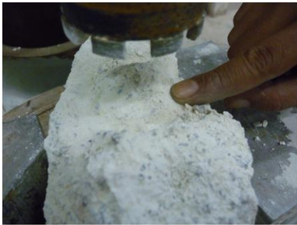
Fig. 5 The dry sample was disturbed partially during use coring apparatus to prepare it for the direct shear test.
