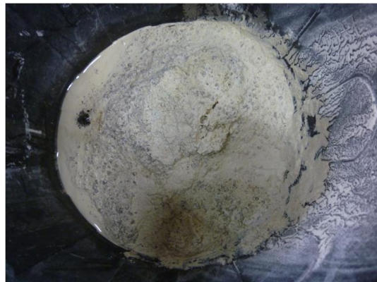
Fig. 9 The samples fully destroyed after submerged in water for less ten minutes.
