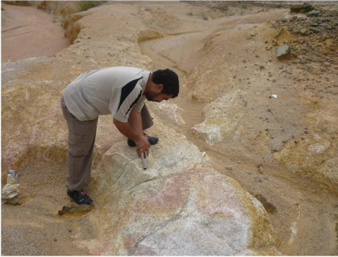
Fig. 4: Measured surface hardness of older alluvium by Schmidt (rebound) hammer.
